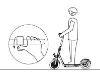
3. When the electric scooter is sliding, the other foot steps on the pedal. After the feet step on the pedal, slightly press the throttle (speed above 3km/h will start the throttle).
