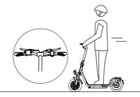
4. Release the throttle can slow down the speed, and automatic energy recovery system can help to slow down. Emergent brakes need to pull the handle brake on the left side.
