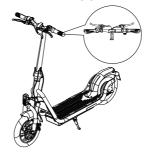
3. Use the hex wrench in the mounting box to lock the screws on both sides
