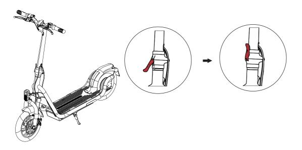
1.Fasten the scooter standpipe and fold out the kickstand
